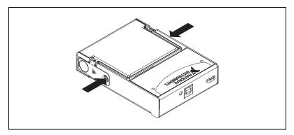
Figure 5. Locking Module into Place
